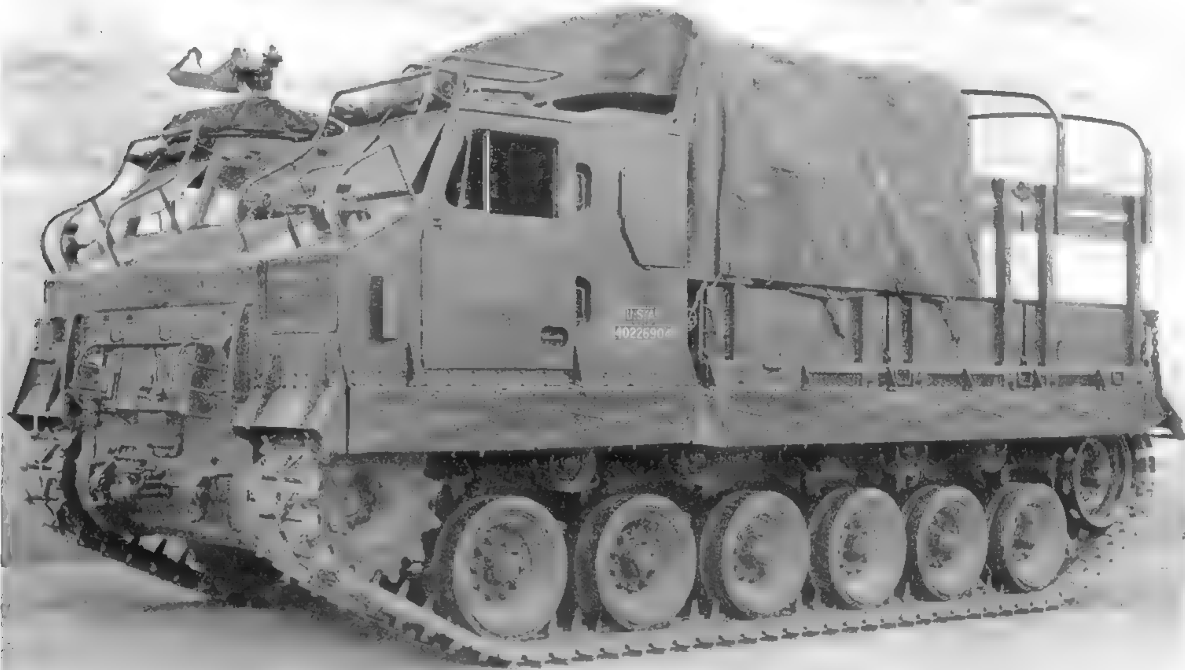
Although this vehicle is not so fitted, a bulldozer blade attachment was available for the G-252 M8A1 tractors. This was useful when preparing the emplacements for the weapons the tractors towed. (U.S. Army photo)
